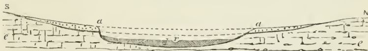
Section in the Valley of the Seine. a a , high-level gravels; d , valley gravels; r , present river-course; e e , chalk-rock in situ .
